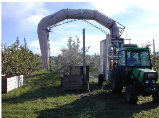
Fig. 2.5: RÉCUPAIR sprayer for orchard – spray recovery sprayer (SRS)
