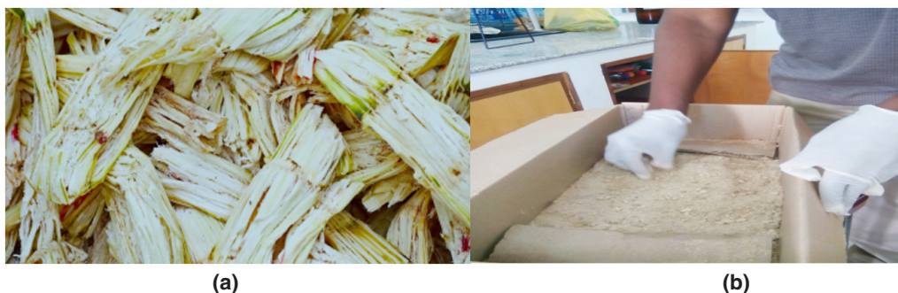
Fig. 2: (A) SCB collected from local sugarcane juice vendors. (B) SCB powder after processing.
