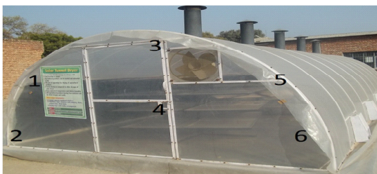
Fig. 1: Position of various thermometers inside the STD.
