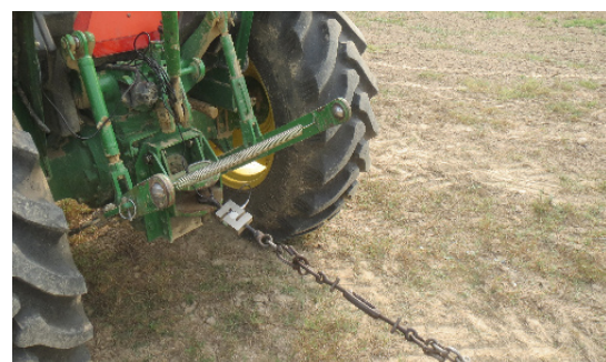
(b) Position of S-type load cell
