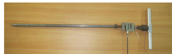
Fig. 5: Hand operated instrumented cone penetrometer
