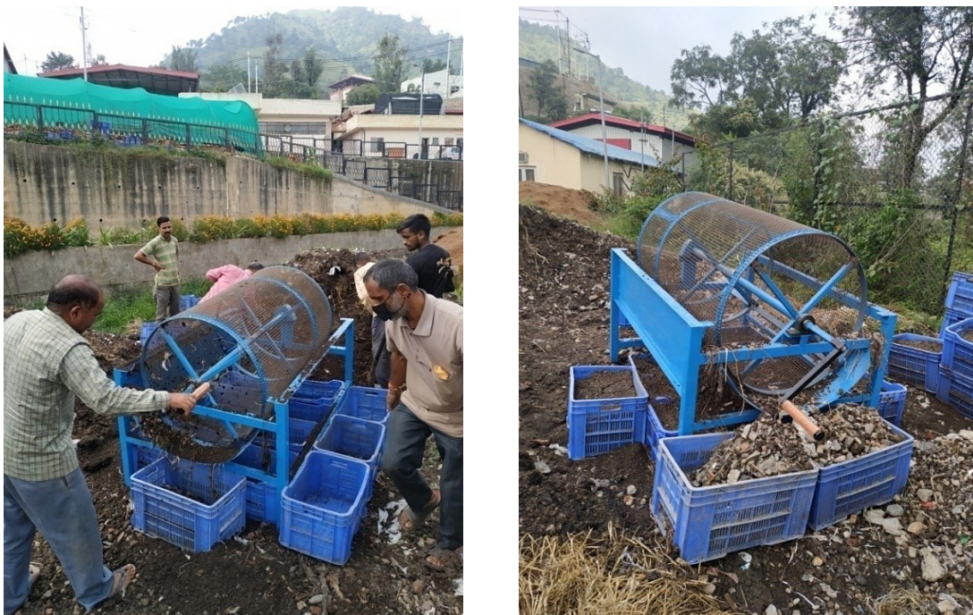
Fig. 2: Farmyard manure sieve a) Rotary sieve in use b) Separated undersize and oversize material from raw FYM
