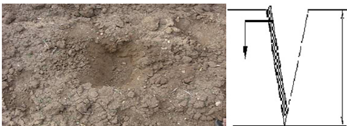
Fig. 2: Soil sample collection point "V" Shaped cutting in the soil in the study area
