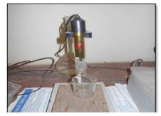
Fig. 3: Electric conductivity meter
