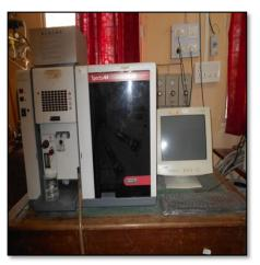
Fig. 1: Atomic Absorption Spectrophotometer
